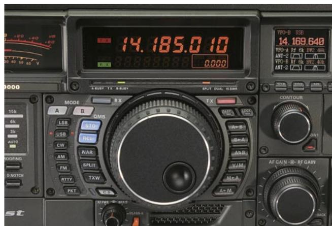
Figure 1 — The main tuning knob, display and the nerve center of the FTdx9000 Contest. The small display to the right shows the frequency of the selected VFO, as well as antenna, roofing filter and bandwidth settings for both VFOs and graphical representations of current roofing filter, bandwidth and shift settings.
