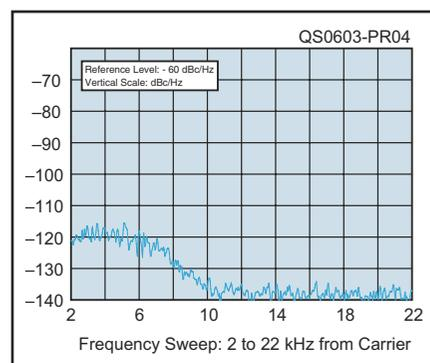
Figure 4 — Worst-case spectral display of the FTdx9000 Contest transmitter output during composite-noise testing. Power output is 200 W at 14.02 MHz. The carrier, off the left edge of the plot, is not shown. This plot shows composite transmitted noise 2 to 22 kHz from the carrier.
