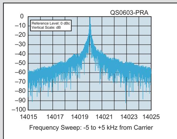
**Figure 5** — Here's an example of a radio with poor keying sideband performance. Note how wide the shape of the signal is compared with the FTDX9000 Contest (Figure 3). This means that the transmitted energy is still fairly strong for several kHz above and below the carrier, with the potential for interference to nearby stations.
