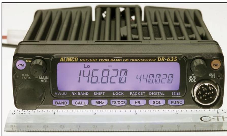
**Figure 6 — The DR-635T is a compact radio with a clear display and large push buttons that make it easy to use.**
