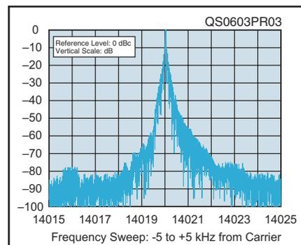
Figure 3 — Worst-case spectral display of the FTdx9000 Contest transmitter during keying sideband testing. Equivalent keying speed is 60 WPM using external keying. Spectrum analyzer resolution bandwidth is 10 Hz, and the sweep time is 30 seconds. The transmitter was being operated at 200 W PEP output at 14.2 MHz.
