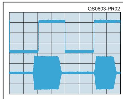
Figure 2 — CW keying waveform for the FTdx9000 Contest showing the first two dits in full-break-in (QSK) mode using external keying. Equivalent keying speed is 60 WPM. The upper trace is the actual key closure (starting at left edge of plot); the lower trace is the RF envelope. Horizontal divisions are 10 ms. The transceiver was being operated at
